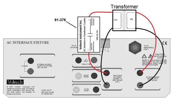
The AC Interface to Transformer Coupler Assembly (91-376) is to be connected in-line with the Secondary output (+) of your step-up transformer and the "Input from External Source (+)" connector on the AC Interface as shown in the diagram.
