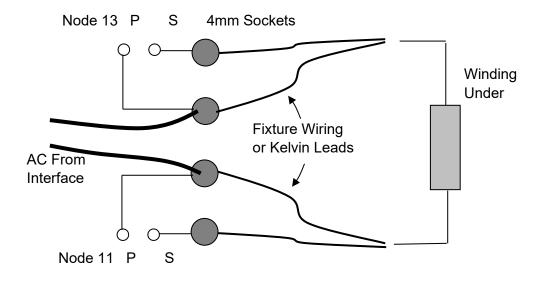
If you are using the universal fixture (# 91-186), the AC Interface output leads can be stacked into the sockets on their required nodes.
