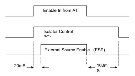
The diagram above shows the signal levels (high or low) and the times between them from when the AT3600/AT5600 asserts its enable signal.
