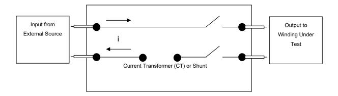
Test current flows from the external source into the fixture and out to the winding under test via an isolation relay.
