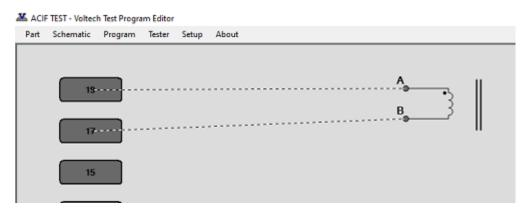
4, Add a VOCX test, with the same 19/A and 17/B nodes used for BOTH Energised and Measured terminals
