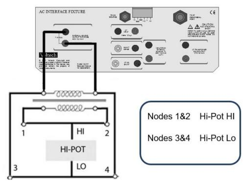
Newer versions of the AT EDITOR will detect violations to this rule and warn you. In most cases, simply reversing the HI LO nodes on the HPAC HPDC tests will resolve this conflict. As the choice of HI / LO for HIPOT testing is arbitrary it will not affect the low current measurement made during a HIPOT test
